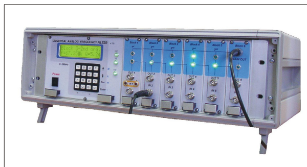
Fig.12 Resulting realization of digitally controlled analog filter unit
