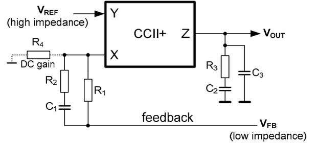
Fig. 7. Second generation current conveyor (CCII) based PID controller.
