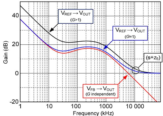
Fig. 5. Comparison of transfers  $V_{REF}, V_{FB} \rightarrow V_{OUT}$  ( $R_1 = 813 \Omega, R_2 = 390 \Omega, R_3 = 2.25 k\Omega, C_1 = 4.51 nF, C_2 = 2.42 nF, C_3 = 100 pF$ , design from [6]).
