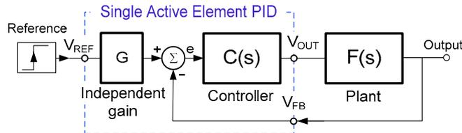
Fig. 1. Structure of SISO closed-loop system with single active element PID controller  $C(s)$ .
