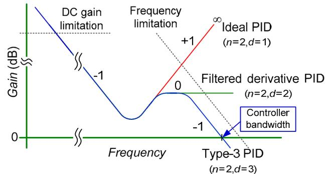
Fig. 2. Frequency transfers with indicated slopes of ideal, filtered derivative and type-3 PID controller.
