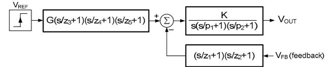
Fig. 4. Block scheme of operational amplifier based controller from Fig. 3.
