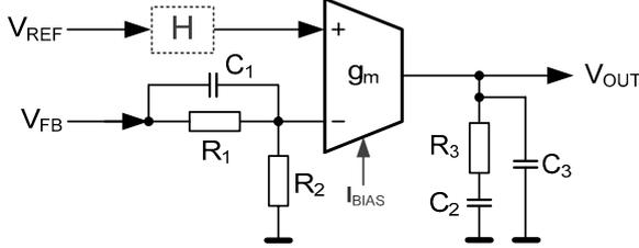
Fig. 6. Controller with operational transconductance amplifier.
