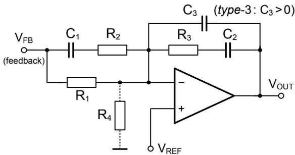
Fig. 3. OpAmp based Controller.  $R_4$  is optional resistance related to  $G$ .
