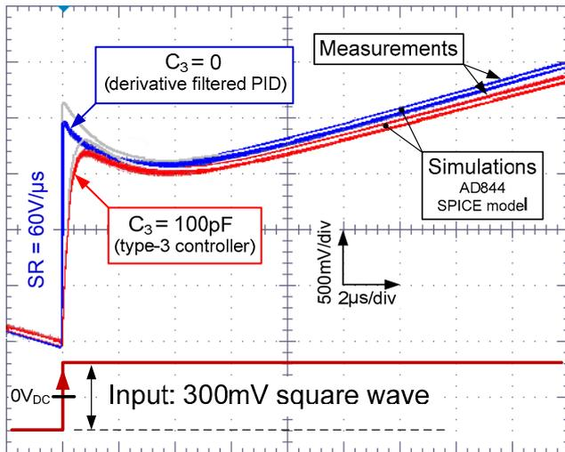
Fig. 8: Measured transient responses of Fig. 7 controller.
